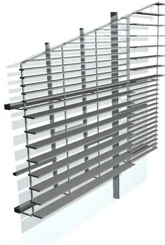
Composition of the External Louvre
